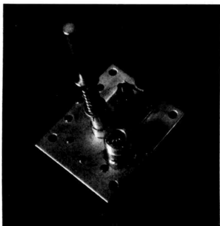
Front view of the cathode partition. Notch on rear edge provides clearance for plate tuning piston.
