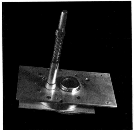
Plate assembly before installation of the cathode cavity.
